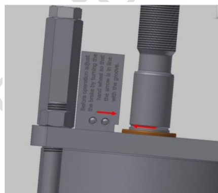
< Figure 1 : Arrow and groove on the chain wheel band brake, here not in line >
