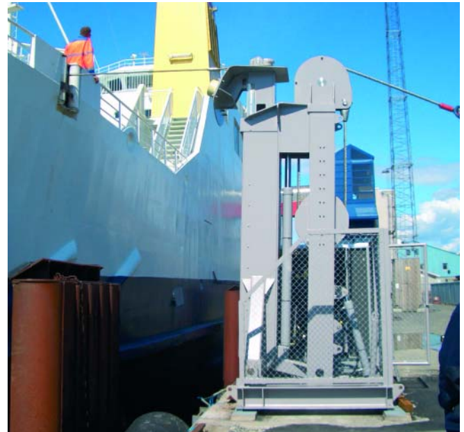
Bollard returned to vertical position and winch is tightened. The vessel is now secured
