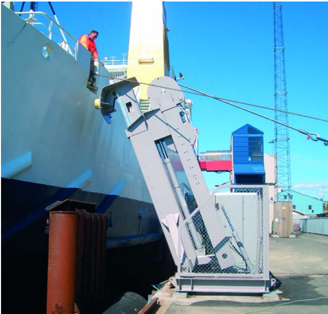
Bollard tilted towards the ship side for connection of wire loop
