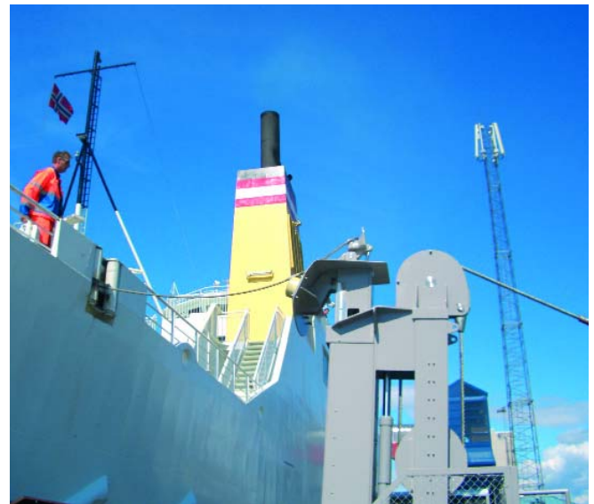
Bollard is tilted and wire loop is free to be pulled back on deck. Vessel departs
