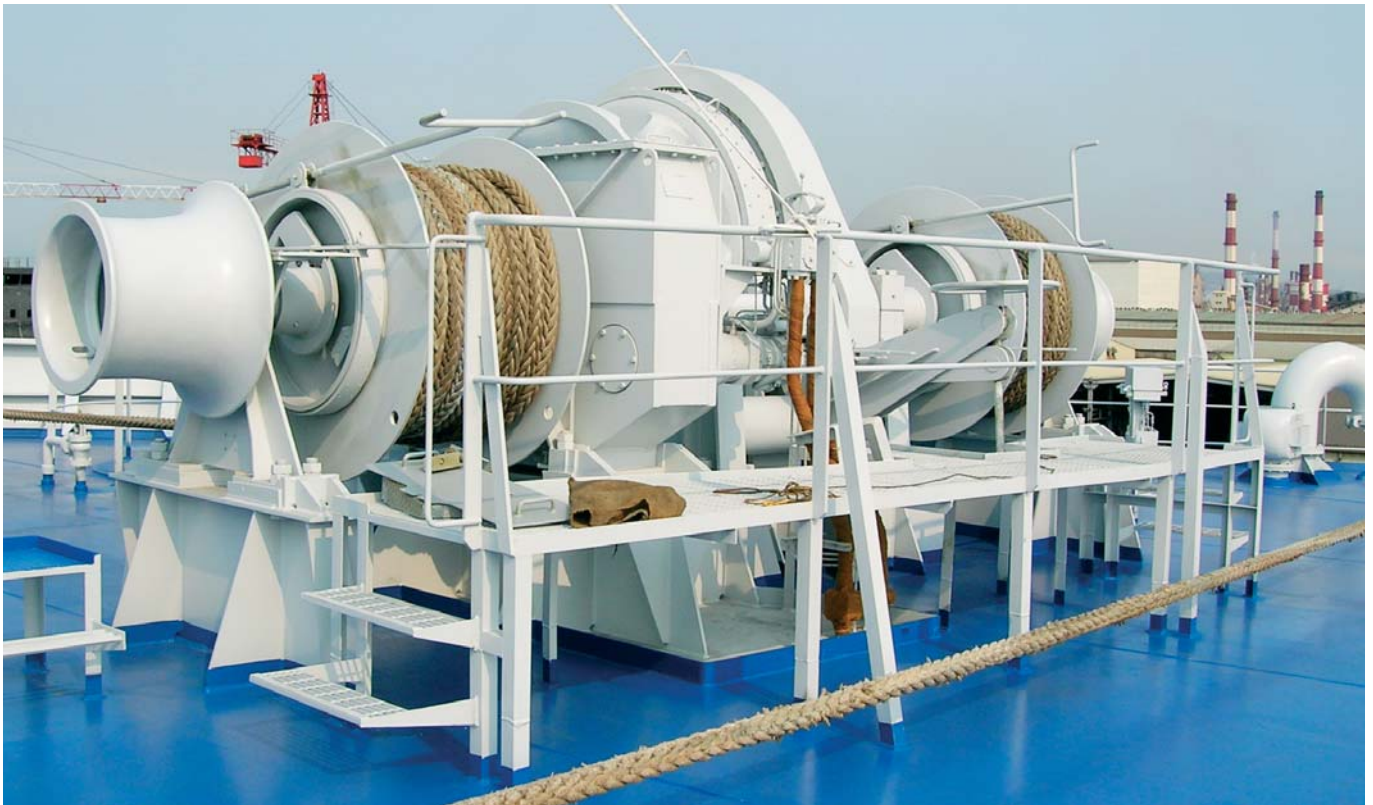
Above: TTS anchor/mooring winch on a 205,000 dwt bulk carrier built at CSBC, Taiwan. Below: TTS cable lifter in production
