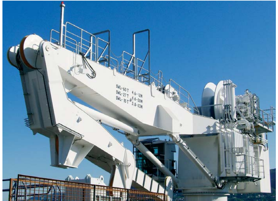
Above and below: the 60-tonne AHC crane under test conditions at TTS workshops, Norway
