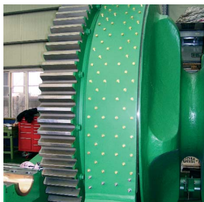
Above: TTS anchor/mooring winch on a 205,000 dwt bulk carrier built at CSBC, Taiwan. Below: TTS cable lifter in production
